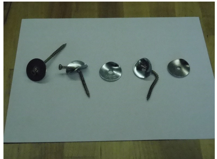
The far left is what they should look like – undamaged.
